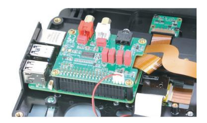
Some HAT boards come with pass-through holes. In such cases, you can use GPIO stacking headers, which allow the pins to extend through the HAT and enable connection of the display power cable.
