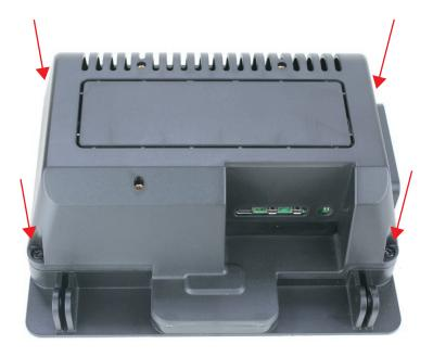
If using the port cover parts, the port cover is positioned between the front part and the back cover as shown below.
