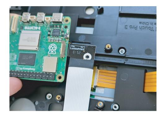
Secure the Raspberry Pi to the case using the four gold screws. Connect the display ribbon cable and the camera cable to their corresponding ports on the Raspberry Pi. Then, attach the display power cable to the GPIO header as shown in the diagram on the right
