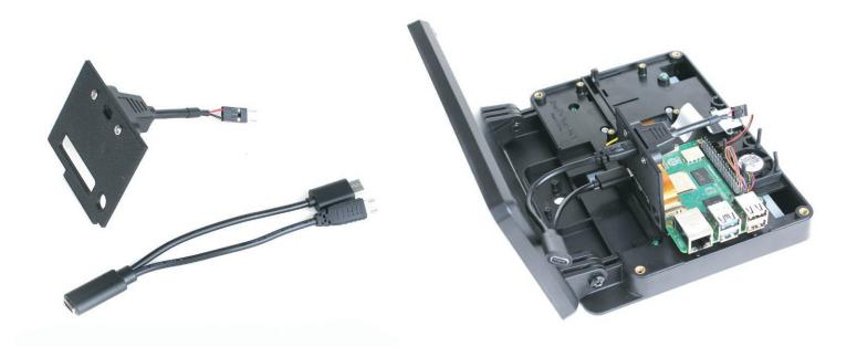
Position the lower panel around the Raspberry Pi connectors as shown below. The panel shown is for the large back cover; a shorter version is included with the small back cover. This panel is optional—the case can be assembled without it.
